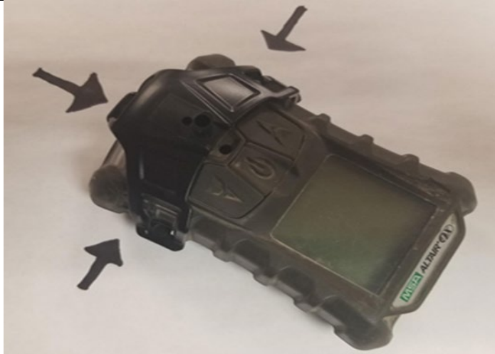
MSA monitor with Calibration cap attached
